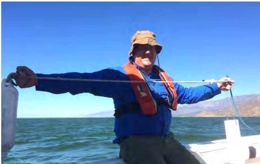
Figure 17. A makeshift drogue was inserted between the tail of the streamer (about 4 m behind it) and the tail buoy in order to minimize the undulation of the streamer while under tow. The tail buoy is at left, and the drogue, a plastic tube containing 2 lb of lead weight, is at right.
