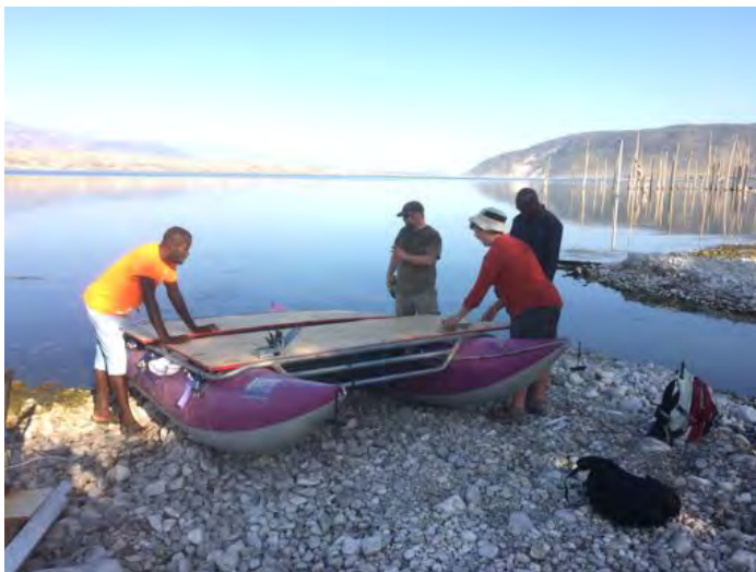
Figure 10. The assembled coring platform, the "cataraft". The gap between the two sheets of plywood is just enough for lowering and recovering the Bolivia corer.
