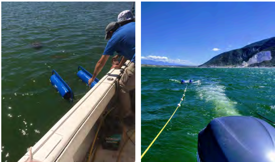
Figure 18. Left: BubbleGun seismic source is lowered in the water. Right: BubbleGun under tow; the seismic source itself dangles ~1 m below the two blue floats; the streamer is not visible, towing ~90 cm below lake surface.
