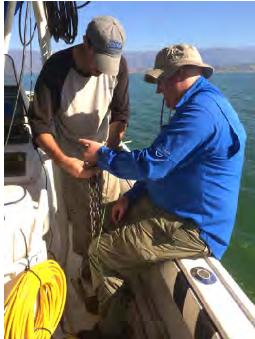
Figure 4. The geophysical equipment was powered by 4 marine batteries connected in a 24 V configuration (top left). These batteries were connected to a UPS and battery charger dual system (top right, and left). A large chain (bottom right) dropped over the side of the boat provided grounding for all the equipment.
