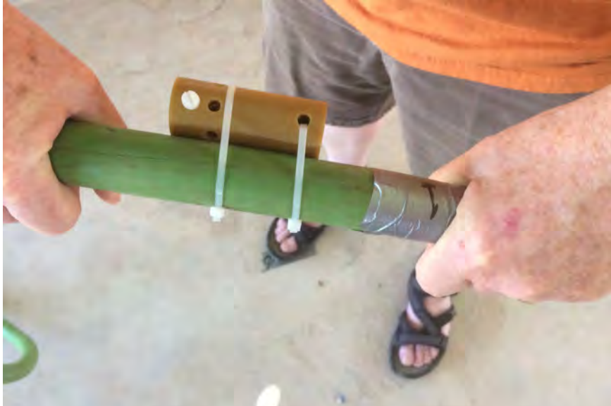
Figure 16. A Star-Oddi pressure sensor within its protective housing, strapped to the seismic streamer. Three such depth sensors strapped near channels 1, 12-13, and 24 internally recorded the depth of the streamer with centimeter accuracy.
