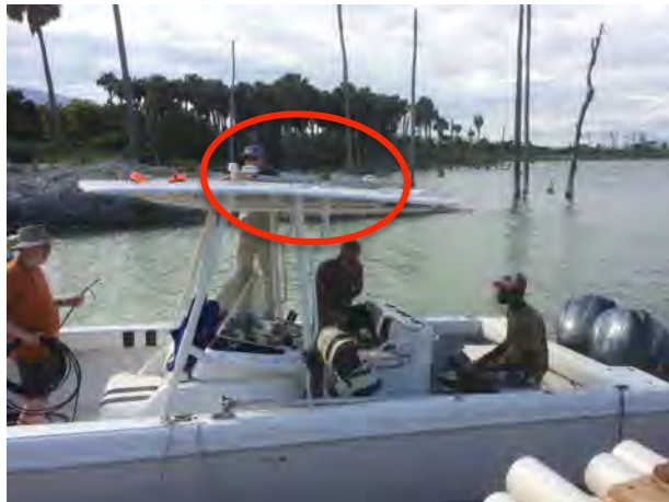
Figure 5. Installing the GPS antennas on the center console canopy
