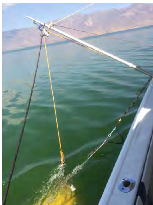
Figure 18. Left: BubbleGun seismic source is lowered in the water. Right: BubbleGun under tow; the seismic source itself dangles ~1 m below the two blue floats; the streamer is not visible, towing ~90 cm below lake surface.
